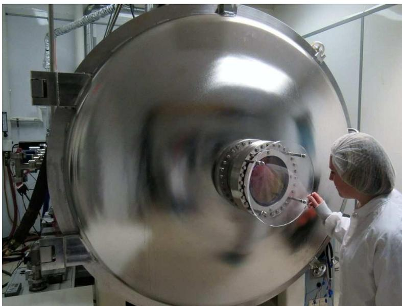
Emily Gleeson peers into a thermal vacuum system, used to test satellite components for temperature and pressure conditions in outer space. Gleeson has recently won a 2018 Amelia Earhart Fellowship.
